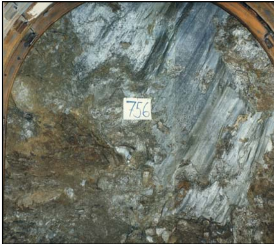
Figure 4. Polished striated surfaces (slickenside), inside the fault breccia found in the exploratory adits. Width of exploratory adit was 2.9 m.
