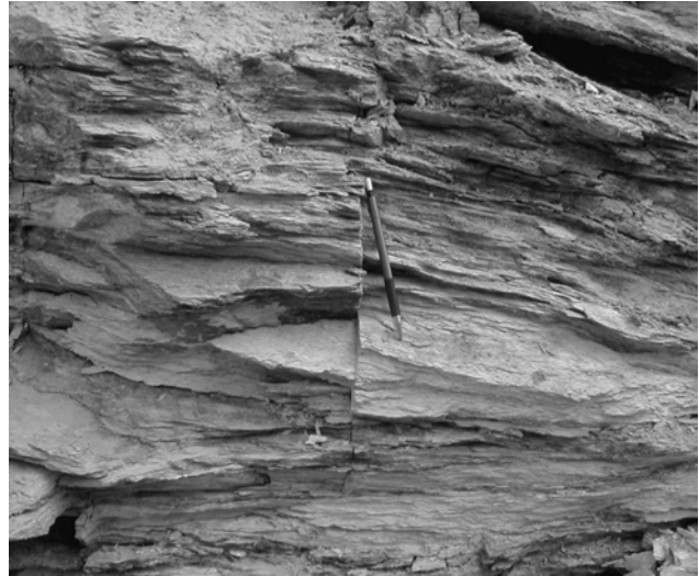
Figure 1. Outcrop of weathered phyllites showing well-developed foliation and a low persistence joint.
